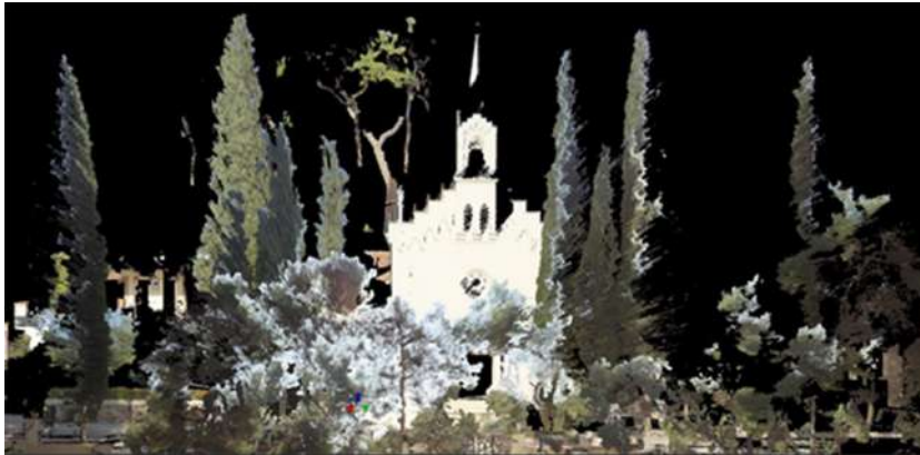
Figure 11. Point cloud externally capturing the church building [Authors]
