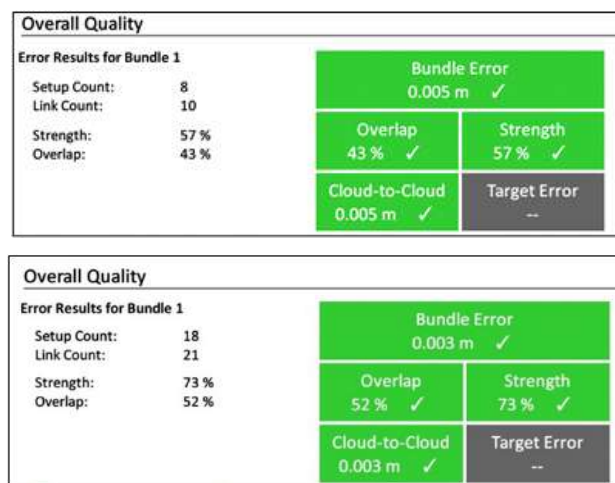
Figure 6. Outside(up) and inside (down) scan cloud model overlap statistics
