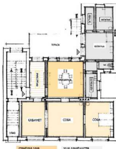
Figure 9. Spatial-functional concept of a salon apartment in the interwar period - Osvald Repić Building (1933), Borivoja Gojkovića 4, Niš, arch. Julian Djupon (Source: Keković, A. (2009). Residential architecture of Niš in the Moderna movement between the two world wars (Doctoral dissertation, University of Niš, Faculty of Civil Engineering and Architecture). Pg.78-79)
