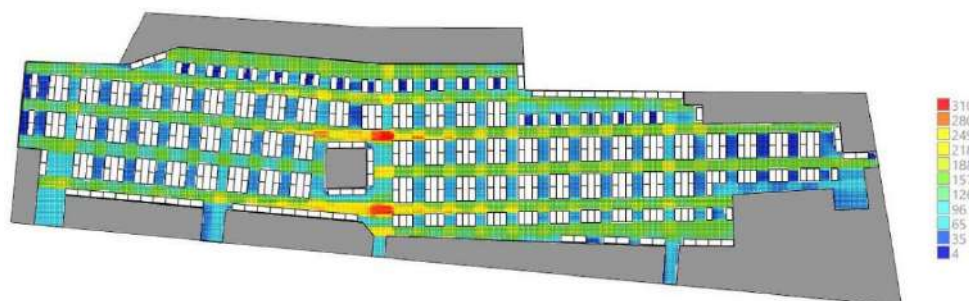
Figure 4. The results of the analysis for the isovist area for the experimental layout of the Futoška Market measured in square meters
