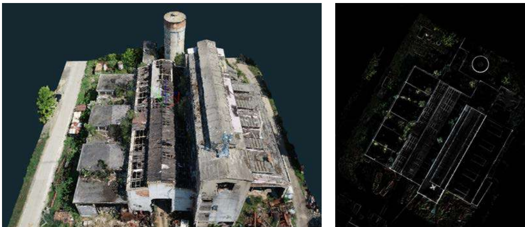
Figure 6. 3D view of the industrial zone model (left view) with automatically generated "X-ray" image of the walls (right view)
