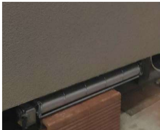
Figure 3. Cross flow fan under the PCM section.
