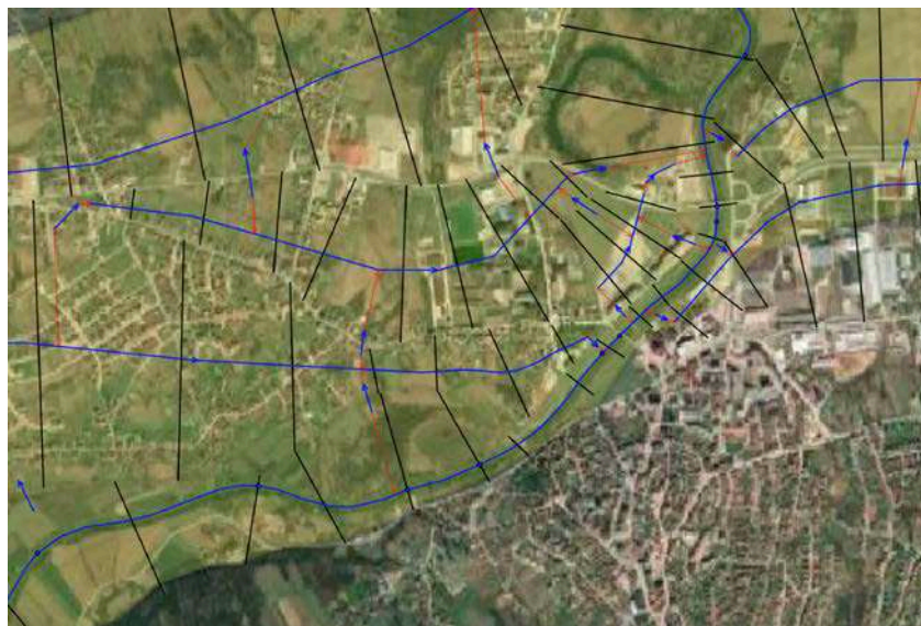
Figure 6. Elements of 1D model for Ukrina River in the city of Derventa (Flow-path centerlines, Cross-sections and Link channels)
