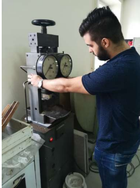
Figure 3. Compressive strength test using Amsler hydraulic press
